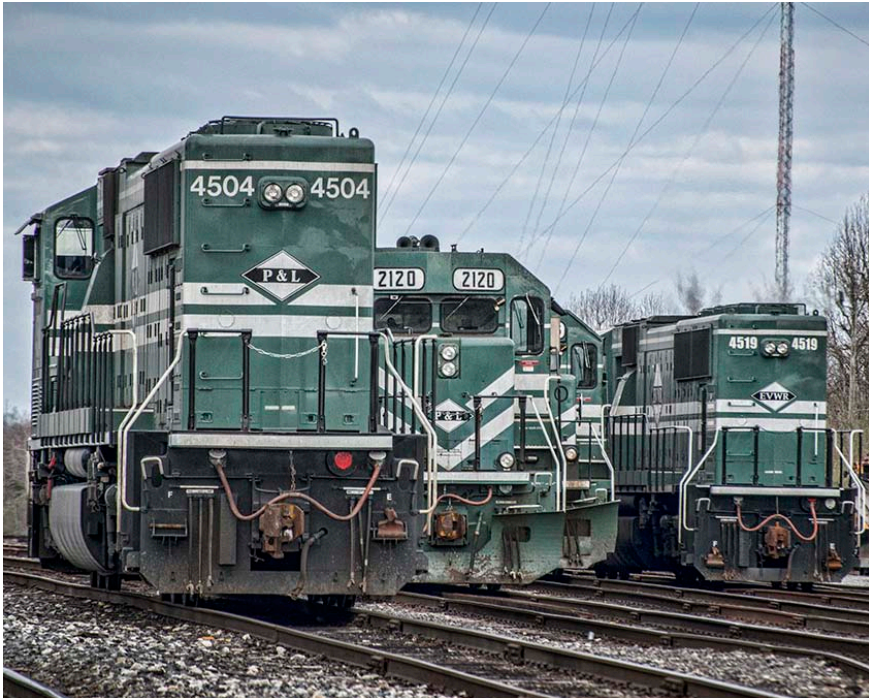
Above: Paducah and Louisville engines 4504 (SD70MAC), 2120 (Road Slug), 3806 (GP38-2 and partly hidden) and Evansville Western Railroad SD70MAC engine #4519 (SD70MAC) sit at West Yards in Madisonville, Ky waiting for their next assignment. -Jim Pearson
